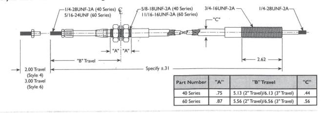
Styles 5 & 7 - Grooved Swivel Fitting with Connection Kit Attachment Fitting
